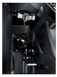
required from the system's electric motor. At slow speed or when stopped, assistance is greatest; assistance is reduced as vehicle speed increases, tightening up the steering. (Photo 15)
