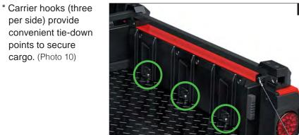
\* 1" square pipes running along the top of the cargo bed side walls and along the back of the bed (cabside) provide easy tie-down points for bungee hooks, and are compatible with the optional KQR accessory mounts (brackets that allow a toolbox or other items
